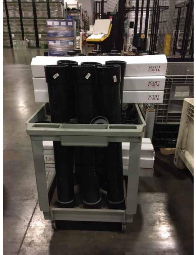
Six storage tubes for 30" cartridge filters
